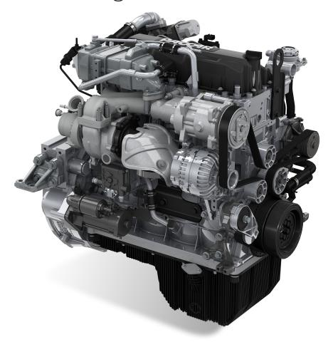
The 4.5 litre Euro 6 PACCAR PX-5 engine uses common rail technology, a turbo with variable geometry and advanced controls for maximum efficiency. In order to comply with the strict Euro 6 emissions requirements, it features exhaust gas recirculation, together with SCR technology and an active soot filter.
